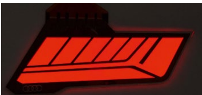
Early generation OLED panel: less than 10 segments. Latest automotive OLED panel: over 600 segments with lit dimensions 56x203mm.
