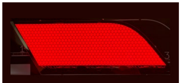
Early generation OLED panel: less than 10 segments. Latest automotive OLED panel: over 600 segments with lit dimensions 56x203mm.
